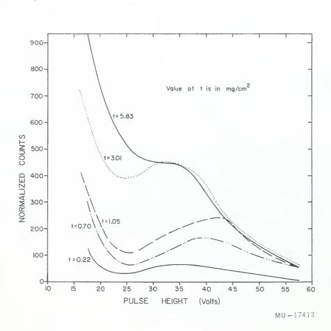
Fig. 3. Experimental differential pulse-height spectra (uncorrected).
